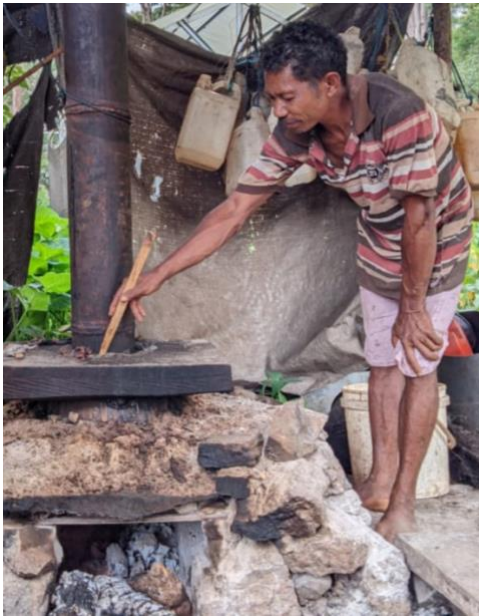
Figure 3. Moke artisan is covering up steam leak
